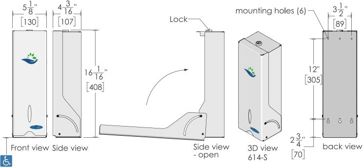
48" (1220mm) Max. height above floor for barrier free installation Floor
