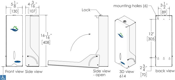
48" (1220mm) Max. height above floor for barrier free installation \$\frac{1}{2}\$ Floor
