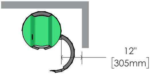
allow clearance to open door when mounting unit in a corner
