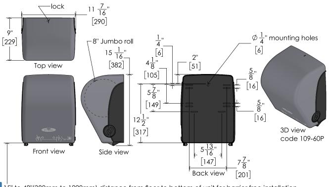
5" to 48" (380mm to 1220mm) distance from floor to bottom of unit for barrier free installation
